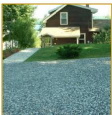
Hard Pack - This is an aggregate stone material that does not wash away as easily as sand and gravel. The lack of fine materials means less sediment erosion.
